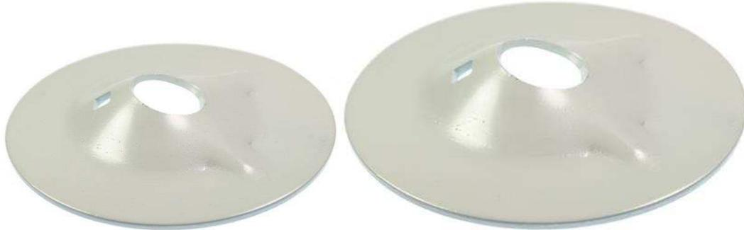
The round bearing plate has a punched-in spherical deformation to fit with a  $\varnothing 50$  mm angle washer and nut for installing Pc-Bolt M27 (combination bolt) and standard rebar bolts  $\varnothing 20$ /M20 and  $\varnothing 25$ /M24 (end anchored and fully embedded). The bearing plate is capable of taking up angle deviations of up to  $30^\circ$ . Pretec stocks two variants.
