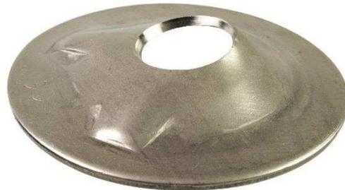
Acid resistant spherical bearing plate used for watertight installation of PE foam, or suspension in concrete elements. Nut on the top (wet) side is sealed with silicon. Nut on the underside (dry side) is torqued. The bearing plate is capable of taking up angle deviations of up to 30°. See PTC 076-15 for installation instructions and principle. Can also be used as standard spherical bearing plate for rock support bolt in corrosive environment.
