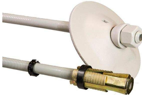
Pc-Bolt M27 combination bolt for rock support. The bolt is used with an expansion shell for immediate work safety support. The bolt is subsequently grouted for permanent anchoring. The bolt is approved by both the Norwegian Public Roads Administration and Norwegian National Rail Administration for use as a combination bolt/rock support bolt in tunnels.
