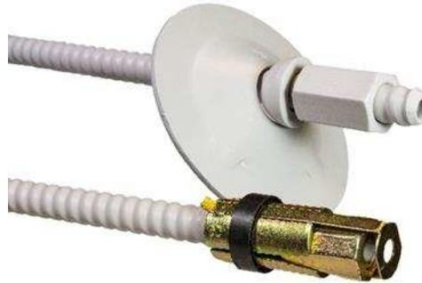
Pc-Bolt R27/12 combination bolt for rock support. The bolt is used with an expansion shell for immediate work safety support. The bolt is subsequently grouted for permanent anchoring.
