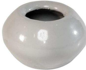
Half ball for use with spherical/triangle bearing plate to achieve a good transfer of forces with angular deviation of the bearing plate in relation to the bolt. This prevent bending momen on the bolt.
