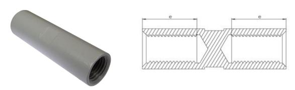
Connecting sleeve for extending ceiling bolts to concrete elements. The connecting sleeve is screwed into the downward protruding rebar bolt or threaded pin from watertight bolt insertion. Well tightened using a key on the key grip of the sleeve.
