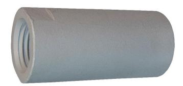
Fully threaded round sleeve for connection of threaded bolts with Pc-Coat™ (HDG and epoxy powder coat). Tensile strength of connector exceeds minimum tensile strength of thread rod of grade 8.8 acc. to ISO 898-1. Threads are oversized to secure correct fit.
