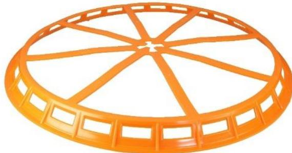
Spacer ring for bolts in dimension M16-M20. Spacer is mounted onto bolt after the front plate has been installed. The spacer is followed by the reinforcing mesh and reinforcement fitting and provides a 25 mm distance between the PE foam / membrane and the reinforcing mesh.
