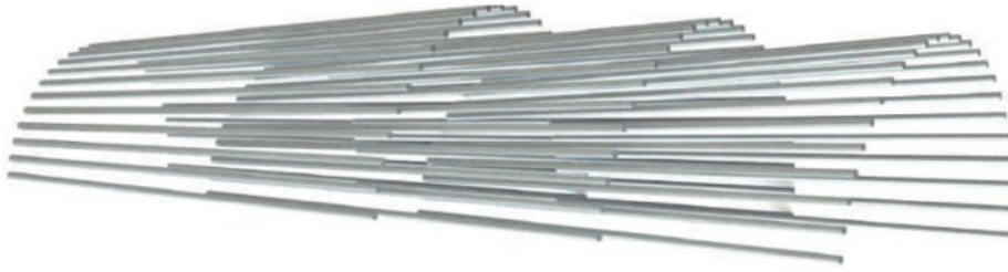
Figure 1: Pipe umbrella illustration
