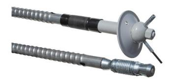
FinBolt™ Gen.2 with integrated packer and expansion sleeve in PC-Coat ensures tightness and prevents water intrusion. The bolt can also be used as a traditional combination bolt. It is used for sealing water-carrying boreholes while the expansion sleeve is used for immediate work safety. The bolt is grouted for permanent safety. The new FinBolt™ 2nd generation with steel tube ensures a higher level of reliability, work safety, waterproofing and safety for correct grouting.
