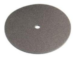
Round PE foam gasket for use between steel plate and membrane in tunnels. Gasket is a vital component for watertight bolting connections. Norwegian road authorities (Statens Vegvesen) report 510, *Gode løsninger for vann- og frostsikring i tunneler*, gives guidance for different solutions for water proof bolt connections. The book also has assembly drawings showing of mounted rubber gasket together with bolts and sleeves.
