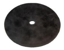
Round rubber gasket for use between steel plate and membrane in tunnels. Gasket is a vital component for watertight bolting connections. Norwegian road authorities (Statens Vegvesen) report 510, *Gode løsninger for vann- og frostsikring i tunneler*, gives guidance for different solutions for water proof bolt connections. The book also has assembly drawings showing of mounted rubber gasket together with bolts and sleeves.
