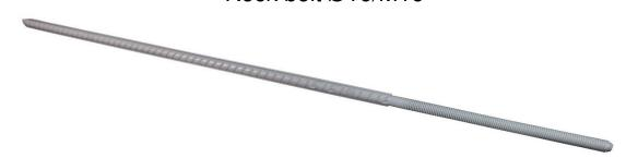
Bolt for fixation of rockfall netting/mesh. The end of the bolt is obliquely cut for improved polyester mixing. For grouting use of retainer  $\emptyset$ 16/22-27 is recommended. Threaded end has a large bevel for easy installation.
