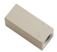
Fully threaded square sleeve for connection of threaded bolts with Pc-Coat™ (HDG and epoxy powder coat) in grade 8 and below according to ISO 898-1. Minimum tensile strength of sleeve is higher than for threaded rod grade 8.8 with corresponding thread dimension according to NS EN ISO 898-1. Threads are oversized to secure correct fit.
