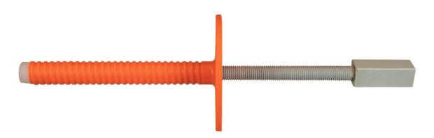
Pretec KS-anchor, is used as a watertight penetration through membrane behind in-situ concrete lining. Anchor is delivered with pre-assembled threaded rod for quick mounting by means of two component anchor glue in shotcrete or rock. Can also be supplied with M16 coupler or double nut and reinforcement fitting (octopus), and membrane welded to flange. Waterproof up to 100 kPa (10m water column).
