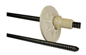
Rock bolt made of glass fiber reinforced plastic (GFRP). Excellent corrosion resistance and well suited for temporary and permanent anchorage. Bolts have a high tensile strength and can be end anchored with either polyester or cementitious grout. Low weight compared to steel which makes it easy for operators to handle. Can be cut to correct length at work site due to it continuous thread.
