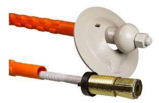
NC-Bolt M22, combination bolt for rock support. The bolt is used with an expansion shell for immediate work safety support. The bolt is subsequently grouted for permanent anchoring.
