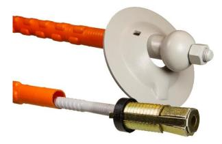
NC-Bolt M20 combination bolt/rock support bolt The bolt is used with an expansion shell for immediate work safety support. The bolt is subsequently grouted for permanent anchoring. NB! These bolts are delivered with pre-assembled expansion shells and packages are suited for stacking to optimize logistics.
