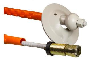
NC-Bolt M24 combination bolt/rock support bolt The bolt is used with an expansion shell for immediate work safety support. The bolt is subsequently grouted for permanent anchoring. NB! These bolts are delivered with pre-assembled expansion shells and packages are suited for stacking to optimize logistics.
