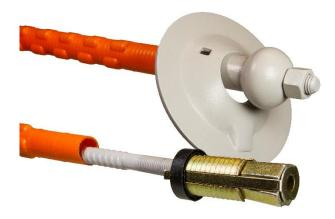
NC-Bolt M33, combination bolt/rock support bolt The bolt is used with an expansion shell for immediate work safety support. The bolt is subsequently grouted for permanent anchoring.
