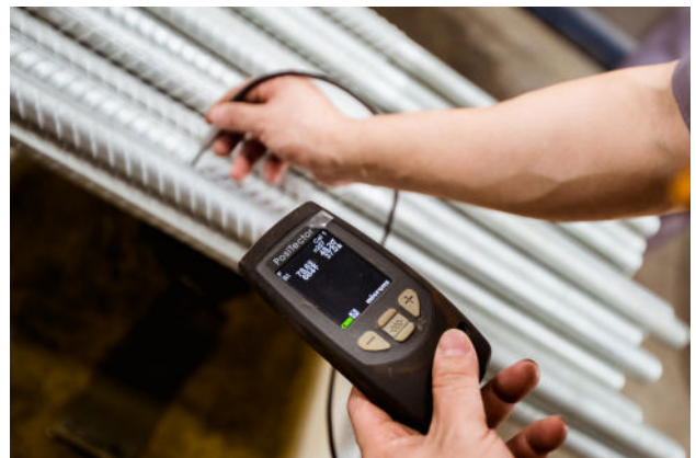
Control of coating thickness
