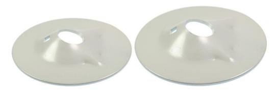
Bearing plate used towards grout head  $\emptyset$ 55 or  $\emptyset$ 67 for installing NC-Bolt M20/M22/M33 (combination bolt). The bolt is end anchored using an expansion shell and then grouted. The bearing plate is capable of taking up angle deviations of up to 30°  $^*$ .
