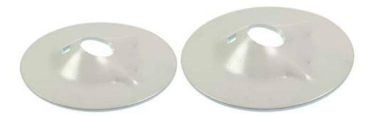
The round bearing plate has a punched-in spherical deformation to fit with a Ø50/63 mm angle washer and nut for installing Pc-Bolt (combination bolt) and standard rebar bolts Ø20/M20, Ø25/M24, Ø32/M33 (end anchored and fully embedded). The bearing plate is capable of taking up angle deviations of up to 30°.
