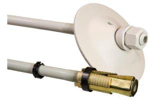
Pc-Bolt M27/15 is a combination bolt for rock support. The bolt is used with an expansion shell for immediate work safety support. The bolt is subsequently grouted for permanent anchoring. Supplied with pre assemled expansion shell. The bolt is approved by both the Norwegian Public Roads Administration and Norwegian National Rail Administration for use as combination bolt/rock support bolt in tunnels.
