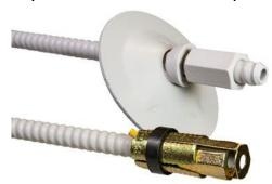
Pc-Bolt R27/12 is a fully threaded combination bolt for rock support. The bolt is used with an expansion shell for immediate work safety support. The bolt is subsequently grouted for permanent anchoring. Supplied with pre assemled expansion shell.
