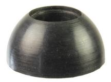
Half ball for use with Ø150 or Ø190 spherical bearing plate to achieve a good transfer of forces with angular deviation of the bearing plate in relation to the bolt. This prevent bending stress on the bolt. The rubber coating aids waterproofing from both sides of the PE foam.
