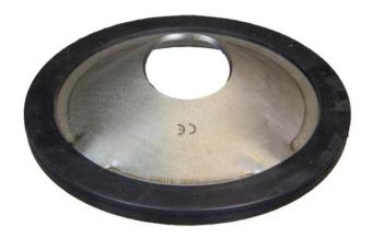
Spherical plate with rubber half ball for use at installation with technical bolts through the water and frost protection vault. Nut and/or rubber half ball on the top side (wet side) is sealed with rubber stopper. Nut on the under side (dry side) is torqued according to specifications for the assembly situation. The spherical plate is capable of taking up angle deviations of up to 30°. Can also be used as standard spherical plate for rock support bolt in corrosive environment.
