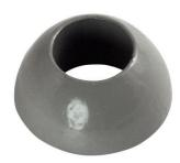
Half ball for use with spherical/triangle bearing plate for load transfer with angular deviation of the bearing plate in relation to the bolt. This bending stress on the bolt.
