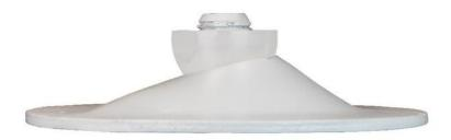
Half ball for use with spherical/triangle plate to give mechanical load transfer from bolt to bearing plate. Threaded half ball is the most compact load transfer system for rebar and combination bolts.
