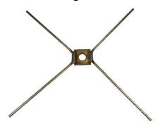
Reinforcement fitting cross stainless steel for use with bolts for PE foam or membrane. The fitting is mounted on the bolt after assembly of the reinforcing mesh, helping to keep the mesh in place during sprayed concrete application.
