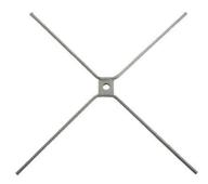
Reinforcing fitting cross for use with bolts for PE foam. The fixture is mounted on the bolt after assembly of the reinforcement mesh, helping to keep the mesh in place during injection molding.
