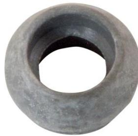
Sealing plug to ensure watertight bolt insertion through back plates. The sealing plug is pre-mounted on the back plate. In order for the sealing plug to function as intended, it is important that the plug is not pulled back and forth on the bolt. If the sealing plug is damaged it can be easily replaced with a new one.
