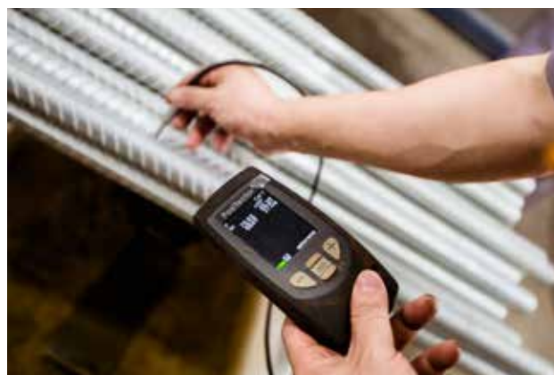
Control of coating thickness
