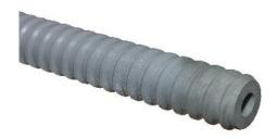
Fully threaded self-drilling anchor bar. For slope stabilization, various mountain rock anchorages also for tunneling. The anchor bars are usually used in demanding geological conditions with mounted drill/clay bit where the anchor bar is drilled in with a simple and flexible joint to achieve the desired length. Can be grouted during drilling or post-grouting.
