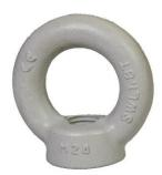
The ring nut is hot-dip galvanized and powder coated. Threaded to fit PC-Coat rebar bolts and threaded rods. Dimensions and capacity according to DIN 582.
