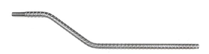
Bolt for suspension of ladders for light fixtures. The bolt is normally mounted in a sleeve / transition sleeve of the same capacity, and is designed to accommodate deviations up to 150mm from the centreline. The equipment is clamped to the bolt or screwed directly onto the thread. For equipent that is to be screwed onto the bolt thread dimension need to specified.
