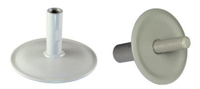
Backplate with welded sleeve provides safe, waterproof bolt penetration through membranes and polyurethane foam. The sleeve is designed to prevent water from following the bolt through the joint. Threads on Pc Coated sleeves are oversized to secure correct fit for bolt with Pc Coat. Corrosion protection according to requirements in N500 from Statens Vegvesen. Can be delivered in stainless steel, se separate data sheet for details.
