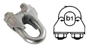
Wire clamps are used to make a loop on the wire, with or without insert inside. In addition, the wire clamp can be used to clamp 2 pieces of rebar bolts in the crossing each other as part of the stiffening or longitudinal to extend the bolts in the tunnel. All components are in HDG to ensure long service life.
