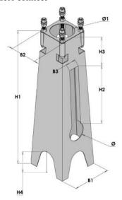
Type 1250 and 1500mm foundations are prepared for 2 alternative C-C-C distances. Alternative C-C-C disance is noted in brackets in table. The foundation is adapted for the insertion of a Ø110mm conduit.
