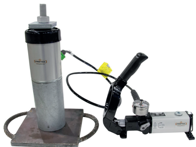
Figure 2: Pull test equipment.
