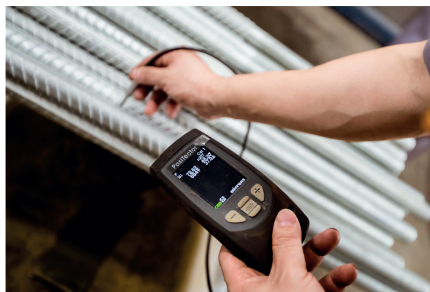
Control of coating thickness
